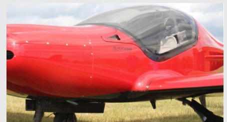
The Blackwing made by Blackwing Sweden AB is an ultralight sports plane made entirely of carbon fibre.
