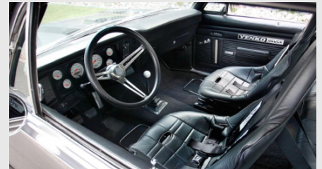
Inside, Björn Morhin modified the US model: He replaced the original bench seat with two separate racing seats.
