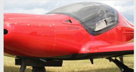
The Blackwing made by Blackwing Sweden AB is an ultralight sports plane made entirely of carbon fibre.
