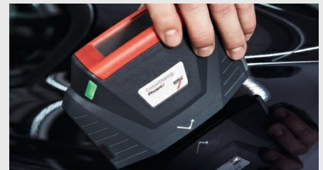
Light and compact: The new ColorDialog Phoenix allows you to measure colours even closer to the damaged area.]
