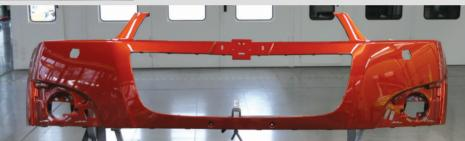
Follow the particular OEM process/guidance on bumper repair. Pay attention to the film build limitations/ sensor requirements. Follow relevant Spies Hecker product TDS's. Please refer also to the Spies Hecker Plastic Painting System TDS – SHPlasticSystem. Refinished plastic car parts should not be washed with a high-pressure jet cleaner within the first six weeks. After this period, the nozzle must be held at a distance of no less than 30cm from the object.
