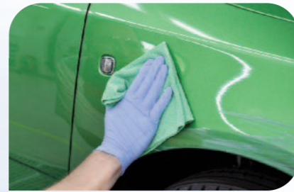
Polish and clean the measurement area close to the damage.
