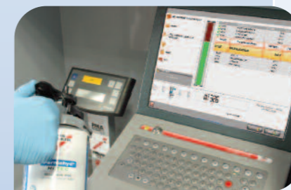
The scale function on the screen aids color mixing and automatically corrects the formula in the event of weighing errors.
