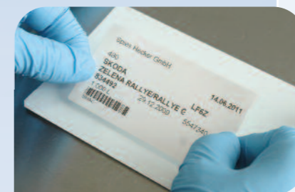
Print out the manufacturer and color formula with a barcode on the label and stick it onto the back of the sample panel.
