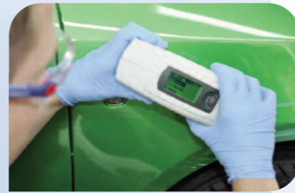
Place the ColorDialog spectro on the cleaned surface and carry out 3 measurements in slightly offset positions.
