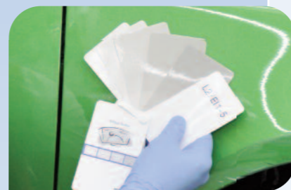
For effect paintwork, determine the coarseness of the metallic paint with the Effect Index.
